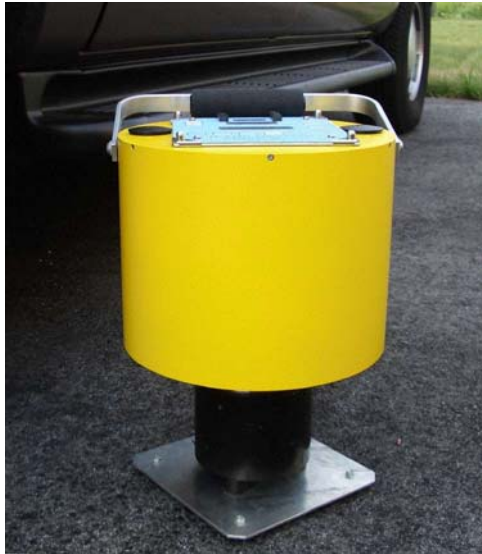
Figure 3: GeoGauge On Verifier Mass H-4140.20
